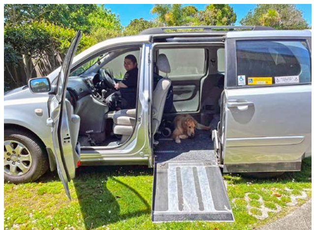
Logan McColl can drive his wheelchair into the driver's seat (above) and uses his left hand for the steering wheel and his right hand for the accelerator and brake.
